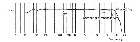
When recording, a bias current according to the tape type used is applied to the recording head as well as the music signal to improve the distortion rate. Furthermore, the extreme high frequency content of a music signal can actually act as bias, adding to the deck's own bias signal to produce over-bias conditions. The result is the deterioration of the high frequency components of the music signal.
